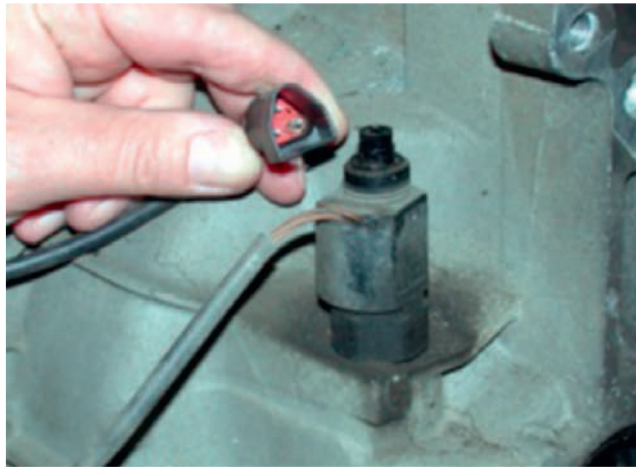
Figure 3.111 Road speed sensor in position
